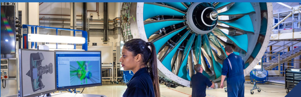
Rolls-Royce's UltraFan™ was part-funded by considerable ATI R&D grants. The engine, first fully tested in 2023 and capable of running on sustainable aviation fuel (SAF), is the world's largest aero engine technology demonstrator, providing both a new engine design and a suite of technologies that can support more sustainable air travel for decades to come. [Credit: Rolls-Royce]
