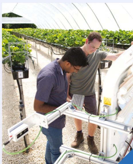
Thorvald Platform testing inside a polytunnel, Riseholme Park (Source: University of Lincoln)
